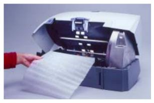
5. Lower the scanner door and press it down firmly until it latches into place.
